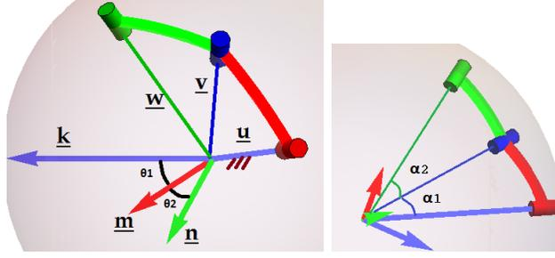
Figure 1: A single link on sphere, and 2R spherical serial
